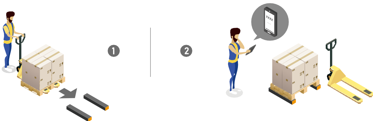
Put cartons or pallet on — open its APP - get weight information on APP
